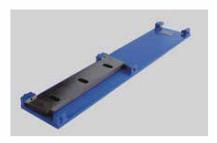
Rotor and stator knives are pre-set outside the machine prior to installation in a supplied fixture. This makes awkward adjustment inside the machine unnecessary.
