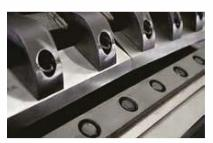
The GSH granulators are available with different rotor options to fit different applications, all rotors feature the V-cut technology creating a high quality regrind.
