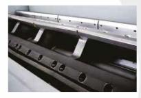
The GSH 1100 series comes standard with wide H-style rotors available with 9,11 or 13 rows of rotor blades ensuring a high quality output.
