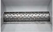
The rotors are equipped with square knives, producing high quality output. The cutters can be turned after they are worn.
