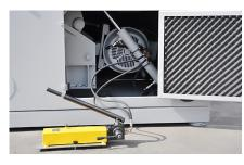
Rotor and stator knives are pre-set outside the machine prior to installation in a supplied fixture. This makes awkward adjustment inside the machine unnecessary. To ensure a safe operation and quick and easy access for cleaning and maintenance, the GSC 500 machine's cutting chamber is opened hydraulically.
