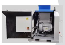
To minimize needed floor space and make the machine easy to move, the control cabinet is integrated into the machine's soundproof housing.
