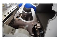
Rotor and stator knives are pre-set outside The machine prior to installation in a dif supplied fixture. This makes awkward adjustment inside the machine unnecessary.
