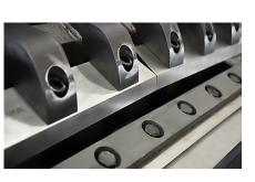
The GSH granulators are available with different rotor options to fit different applications, all rotors feature the V-cut technology creating a high quality regrind.
