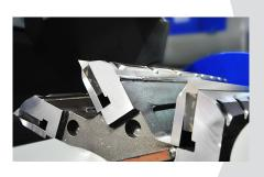
For abrasive applications the GSH granulators can be equipped with rotors with key parts manufactured from highly wear resistant steel as well as welded on hard facing.
