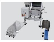
Due to the Quick snap fasteners used on the GSL series machines, the machines can be opened for cleaning and maintenance quickly without the need for special tools.
