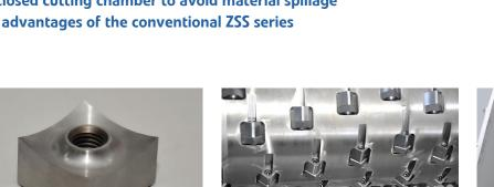
The shredders use concave, ground, square knives producing high quality output. The cutters can be turned after a side is worn out.
