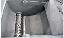
The internal ram design on the ZIS series allows the cutting chamber volume to be increased while keeping a small footprint. The ZIS is ideal for shredding of big volume parts.
