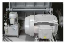
In order to keep the GSC series as compact as possible, motor and hydraulic opening system are integrated into the sound dampening enclosure of the machine.
