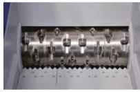
The rotors are equipped with square knives, producing high quality output. The cutters can be turned after they are worn.
