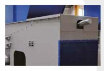
Angled hydraulic pusher to ensure optimal material feeding and ingestion.
