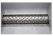
The rotors are equipped with square knives, producing high quality output. The cutters can be turned after they are worn.
