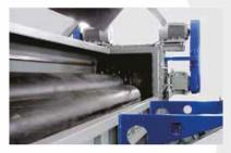
The ZRS pipe shredders are equipped with a special feeding trough sized to take pipes of up to 6 m length. A powerful hydraulic ram forces the pipes into the rotor.
