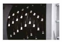
The ZRS shredders use very large diameter flat E-style rotors. The knives are fixed in special knife holders fitted in machined pockets.
