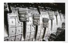
The ZTS and ZTTS shredders are equipped with a large diameter flat rotors with weld on hard facing. The knives are fixed in special knife holders fitted in machined pockets.
