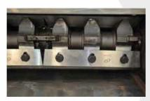
The granulator part uses a sturdy F+ rotor to ensure a good ingestion of the material flow while still being able to handle thicker and heavier particles.
